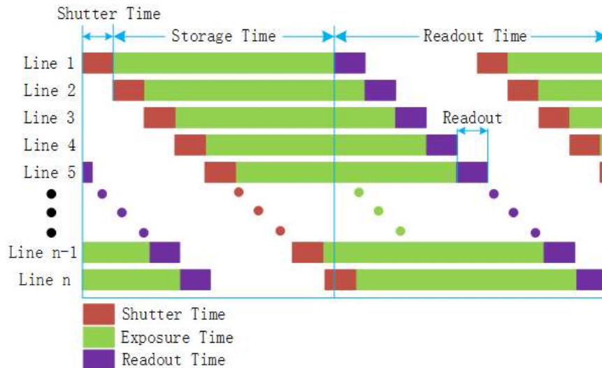
Figure 4-5 Rolling shutter exposure principle
